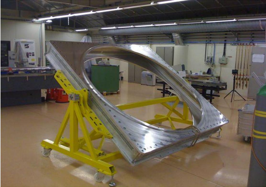
Figure 7: The Straw module 0 frame in the transport trolley.
