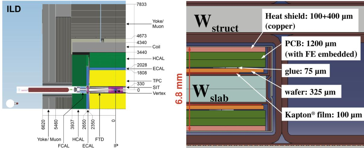
(a) Quadrant view of the ILD with the interaction point (IP) in the lower right corner. Dimensions given are in mm[26]. (b) Cross section through the SiECAL. The silicon layer is labeled 'wafer' and surrounds the W slab[26].
